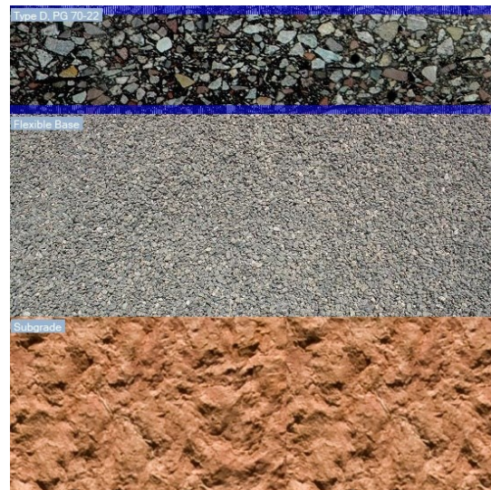
Figure 33. Example of a Conventional AC Pavement Structure.
